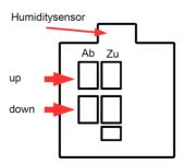
The bottom connecting terminals must be used for operating the SEVi 160DUO MINI ventilation system.
